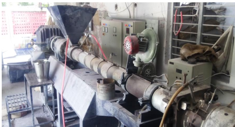
Figure 1: PVC pipe extrusion process
