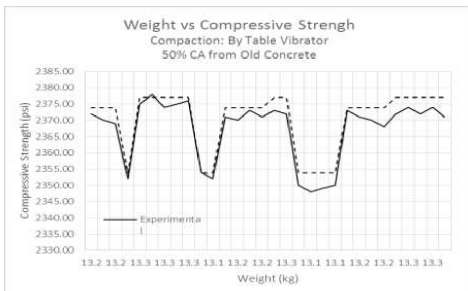
Figure 2: Graphical comparison of experimental and predicted compressive strength (TV)
