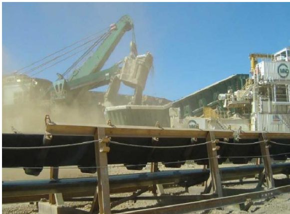
Figure 1: Large Rope shovel loading a mobilizing station (Dewangan et al, 2014).
