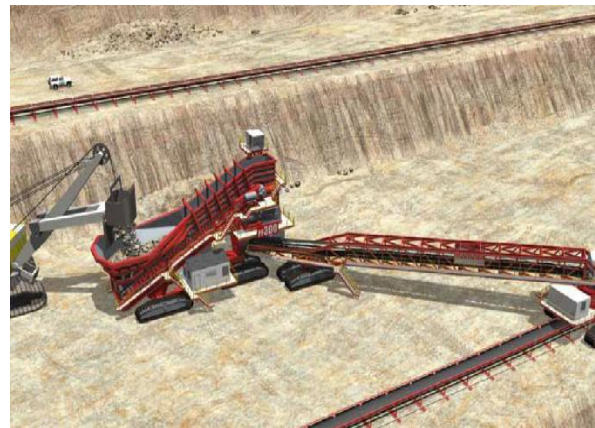
Figure 2: Fully mobile crushing plant on face (Dewangan et al, 2014).
