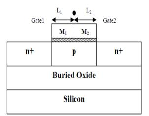
Schematic cross section view of dual material gate SOI MOSFET is as follows.
