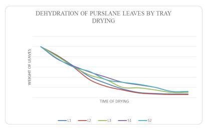
The graph shows that total time taken for drying of leaves in tray drier is 300minutes (5 hours).
