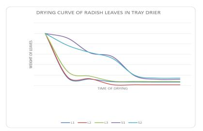
The graph shows that total time taken for drying of leaves in tray drier is 210 Minutes (3.5 hours).
