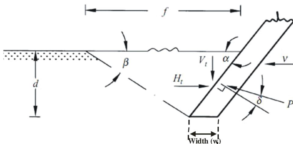
**Figure 1: Schematic diagram of tine in digging position showing the respective parameters:  $f$ , Rupture distance,  $d$ , Tillage depth,  $\beta$ , Soil rupture angle,  $H_t$ , Draught,  $V_t$ , Vertical force,  $\alpha$ , Rake angle,  $v$ , Speed,  $\delta$ , angle of soil metal friction and  $w$ , width of tool (Odey and Manuwa, 2016).**
