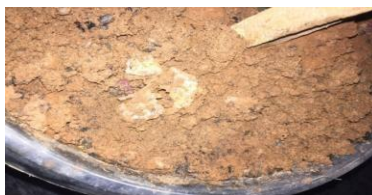
Fig. 11: Biodegraded fabric in soil.
