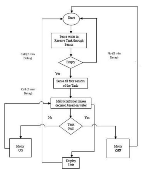
To make the system more easier microcontroller is been used hence the complexity of circuit has been reduced and the design has been simple. Here the water level is sensed by an inverter and input from the sensor unit is taken by a microcontroller. Water pump's action (either ON or OFF) is depended on water status of water tank which is related to input variables. Through a flow chart of whole design is given blow in Fig. 01.
