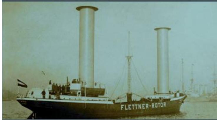
**Figure 2.2: Magnus Flettner rotor (Axis & Turbines, 2014).**
