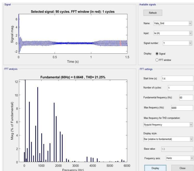
**Figure 17: FFT analysis graph of Frequency Vs Mag (% of fundamental).**
