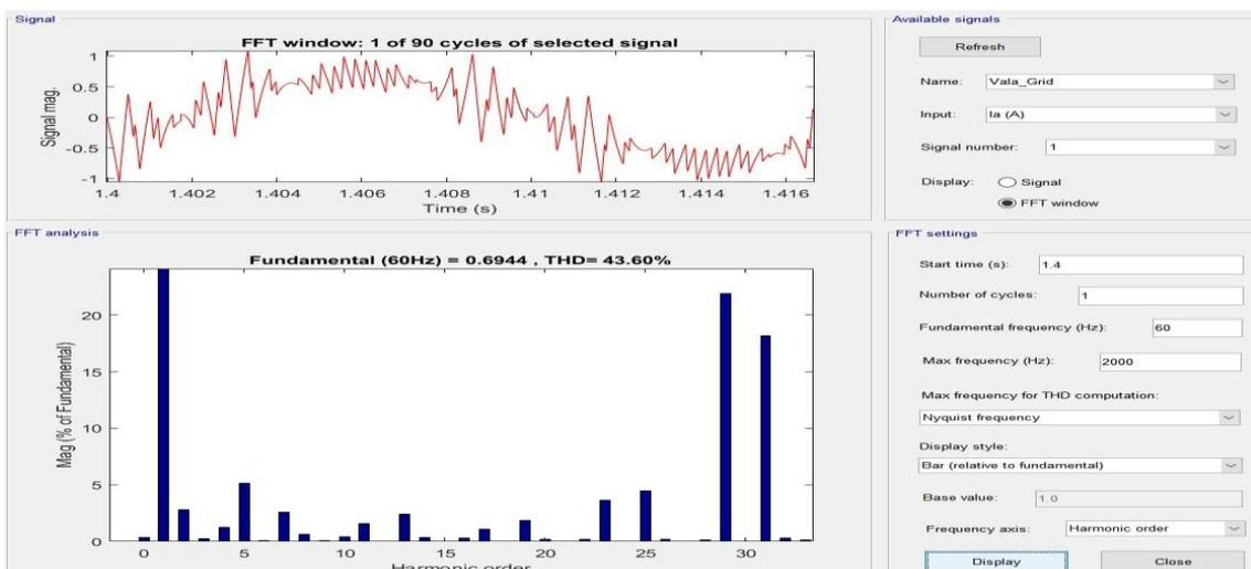
Figure 22: FFT window of signal and graph of Harmonic order Vs Mag (% of fundamental).
