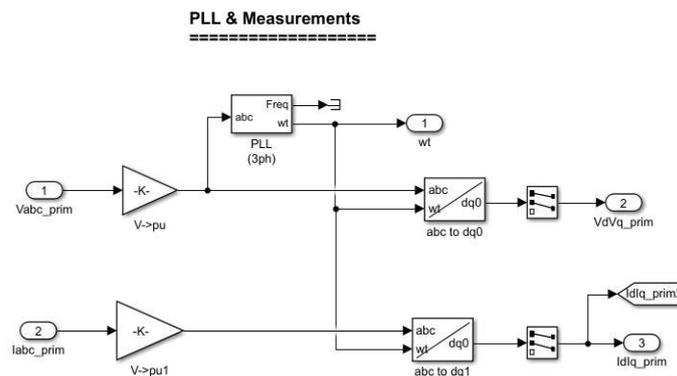
Figure 6: subsystem of PLL measurements.
