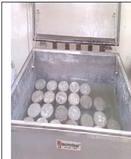
Fig. 2: Specimen in curing tank.
