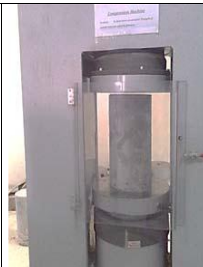
Fig. 3: Specimen testing for compressive strength.
