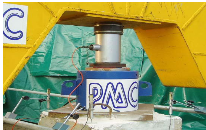
Fig. 3: Example of a Pile load train.
