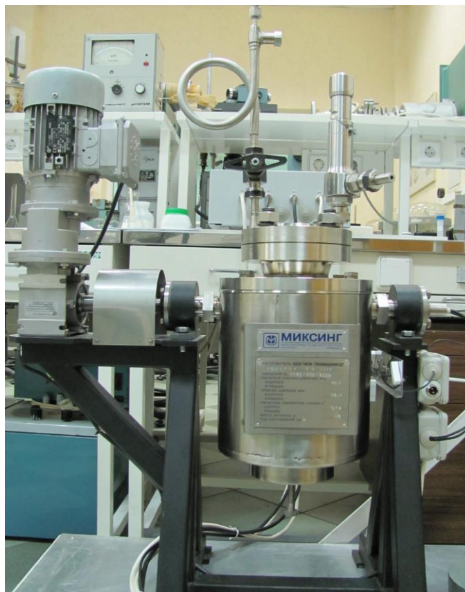
Figure 3: General view of the autoclave reactor setup for synthesis of various nanomaterials under hydrothermal conditions.
