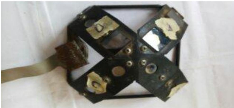
**Plate 1: The Four Quadrant Sensor (light dependent resistors)**
