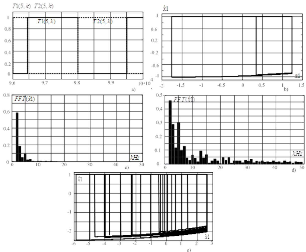
**Fig. 4: Functional graphs of boost converter in CMC mode in steady state at  $t_{ref} = 5$  (a) - output signals of the RS trigger, (b) - limit cycle in the plane  $\tilde{x}1 - \dot{\tilde{x}}1$ , (c), (d) - harmonic**
