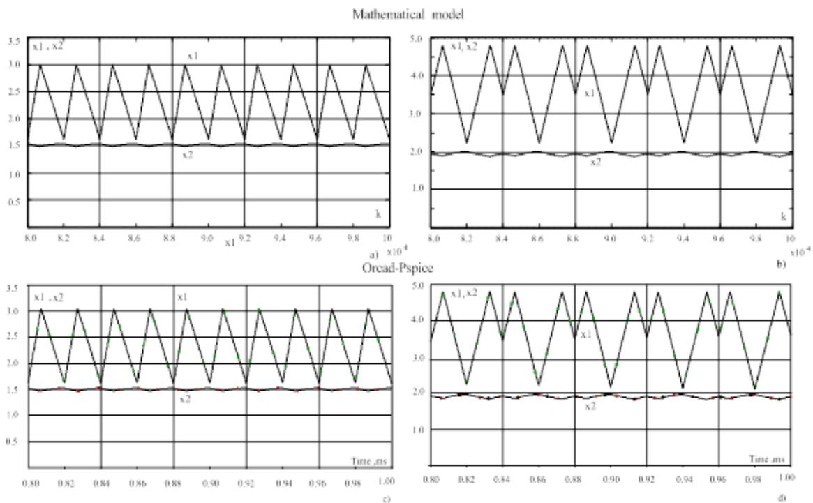
**Fig. 3: Examples of output voltages and input currents in boost converter with CMC-above (a)  $i_{ref}=3$  mode with period  $T_s$ , (b)  $i_{ref}=4.8$  mode with period  $2T_s$ , (a) and (b) – calculated with the proposed model, (c) and (d) – calculated with Orcad-Pspice.**
