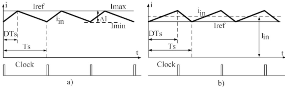
**Fig. 2: Currents diagrams for CMC (a) CMC-above, (b) CMC-bottom.**
