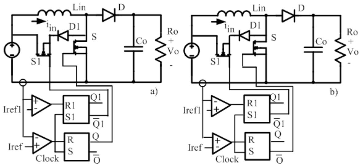
**Fig. 6: Boost converter with synchronization of chaotic process (a) for CMC-above, (b) for CMC-bottom.**
