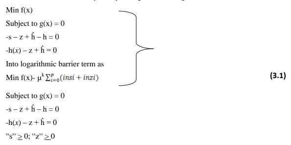
Where, k is the iteration count or number and p the number of interconnected systems for one pool. Solving these equality constraints (Wu, et al 2012, and Ling, 2007), we apply vectors of lagrangian multipliers called Dual-Variables  $^{\Lambda}$ " " $\pi$ " and "v" together with the Newton method
