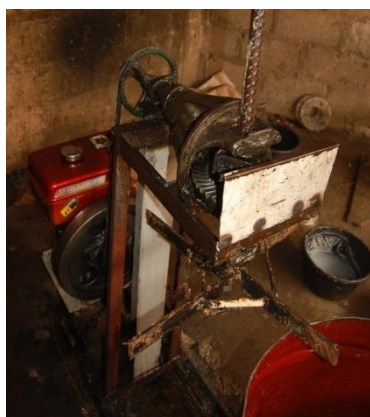
Plate III: Mechanical extractor. Plate IV: Grinding of neem and castor seeds into paste.
