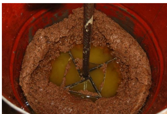
Plate V: Mechanical pressing of neem cake
