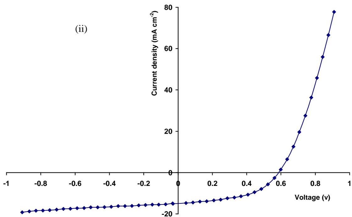
Figure 12 (b): Typical I-V curve of glass/FTO/CdS/CdTe/Au structure, for CdTe deposited at 1500 mV. (i) log I vs V under dark conditions (ii) linear I-V curve under AM1.5 illumination; The rectification factor = 5.39 orders of magnitude at 1 V,  $\eta = 4.0\%$ ,  $J_{sc} = 15.0 \text{ mA cm}^{-2}$ ,  $V_{oc} = 0.58 \text{ V}$  and  $FF = 0.47$ .
