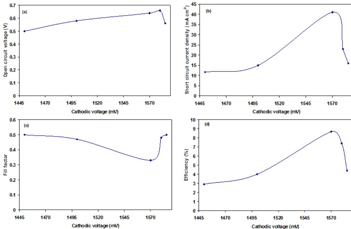
**Figure 13: (a) open circuit voltage, (b) short circuit current, (c) fill factor, and (d) efficiency as a function of CdTe growth voltage.**
