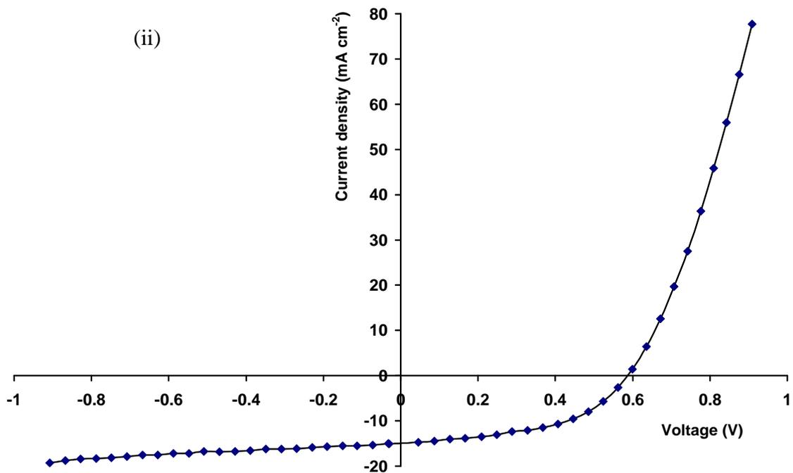
Figure 12 (e): Typical I-V curve of glass/FTO/CdS/CdTe/Au structure, for CdTe deposited at 1585 mV. (i) log I vs V under dark conditions (ii) linear I-V curve under AM1.5 illumination. The rectification factor = 6.4 orders of magnitude at 1 V,  $\eta = 4.4\%$ ,  $J_{sc} = 16.0 \text{ mA cm}^{-2}$ ,  $V_{oc} = 0.56 \text{ V}$  and  $FF=0.50$ .
