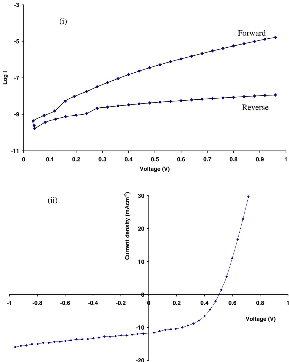
Figure 12 (a): Typical I-V curve of glass/FTO/CdS/CdTe/Au structure, for CdTe
