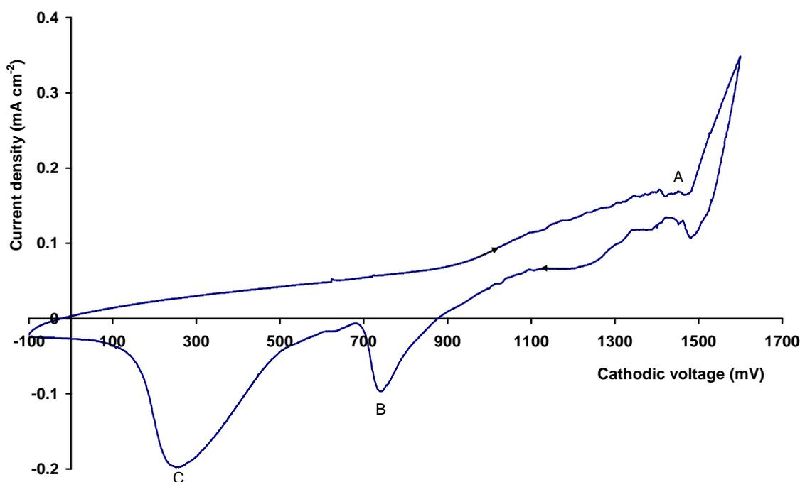
**Figure 1: Voltamogram of CdTe solution containing 0.8 M  $3\text{CdSO}_3 \cdot 8\text{H}_2\text{O}$  and 50 ppm  $\text{TeO}_2$  at  $70^\circ\text{C}$ . The arrows indicate the direction of the potential sweep.**
