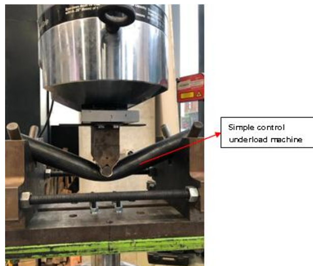
Figure 42: Control specimen under static load.
