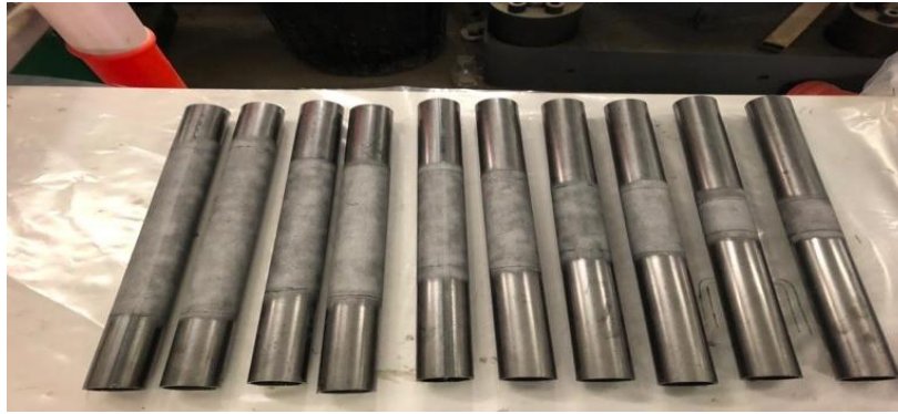
Figure 13: Specimens after clean via sander pester.
