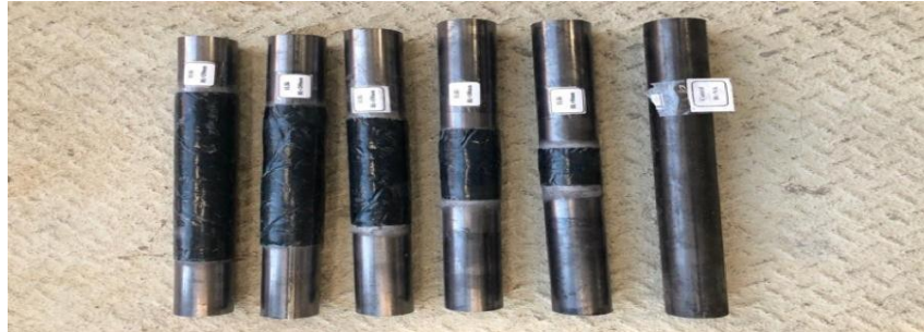
Figure 16: Specimens after wrapping and curing.
