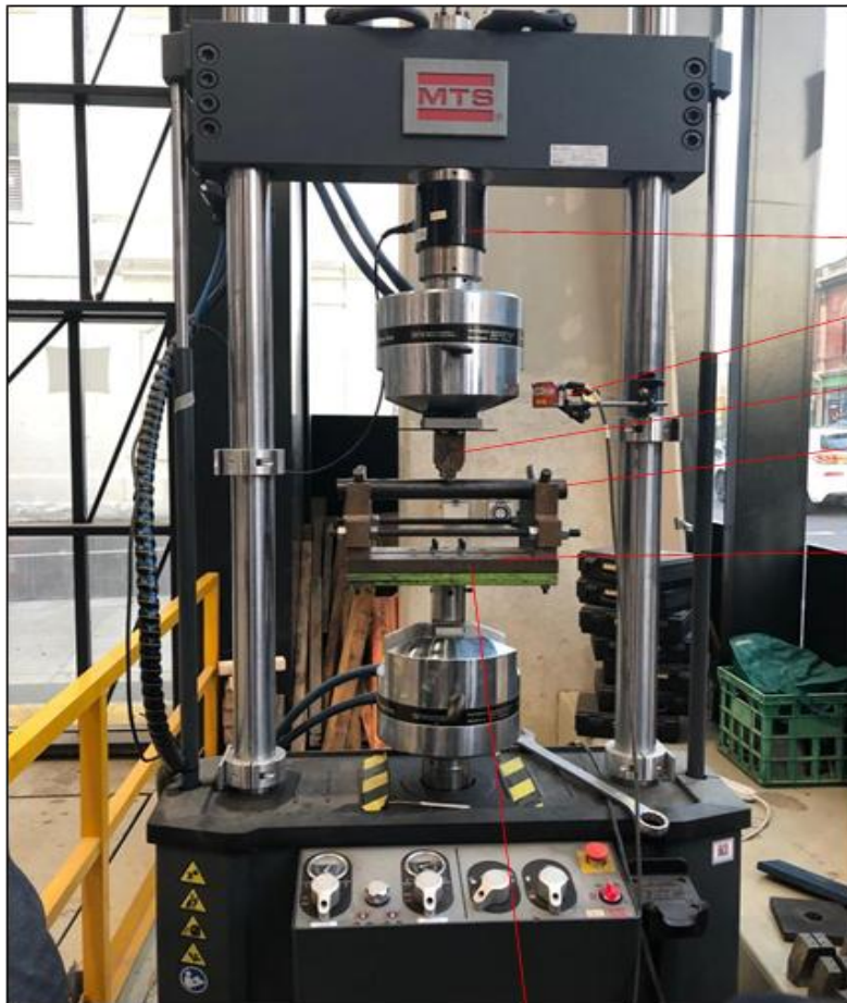
Figure 23: MTS Landmark Servo hydraulic Test Systems for control specimen.
