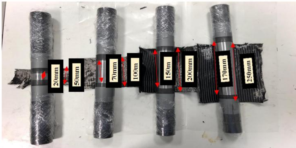
Figure 18: Specimens which lathing before wrapping.
