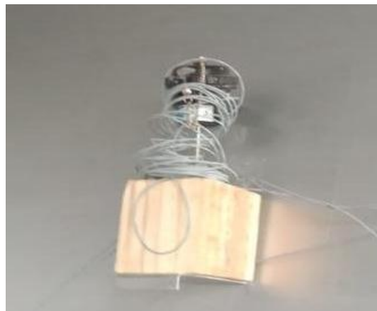
Fig.5. RTD PT 100 sensor fitted in wood core.
