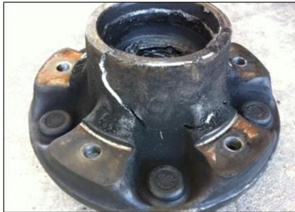
Fig. 1.3: Failure of hub.
