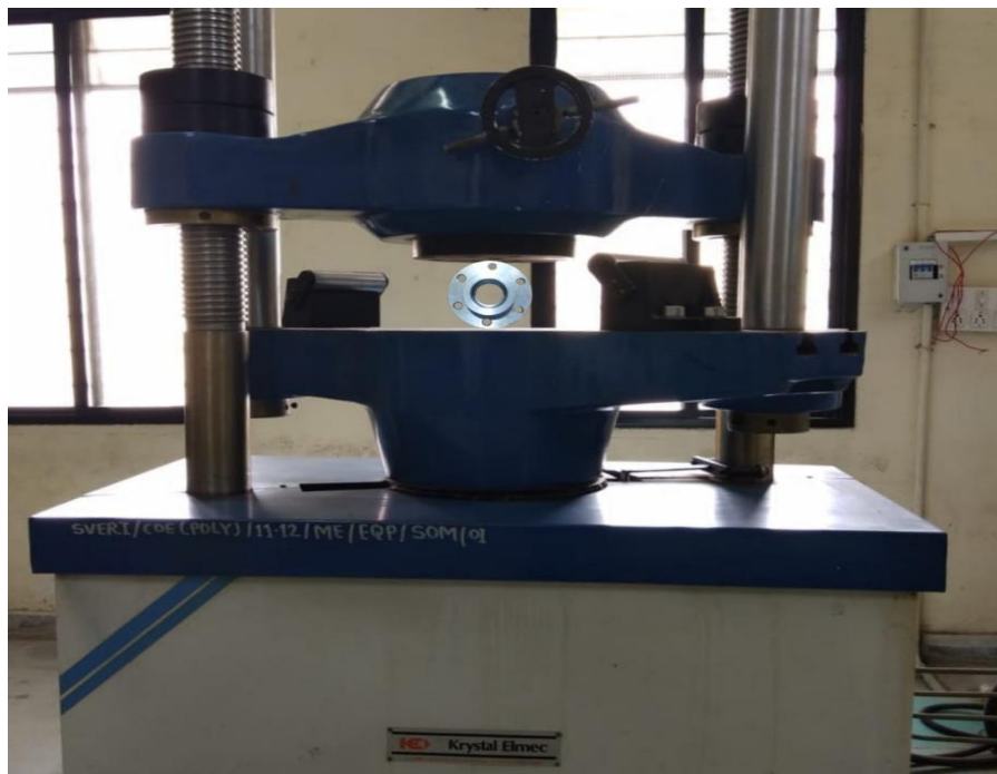
Fig. 8.1: Loading of specimen (MS Hub).
