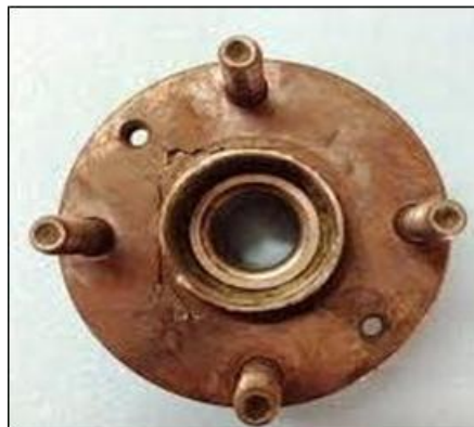
Fig. 1.4: Failure of hub.
