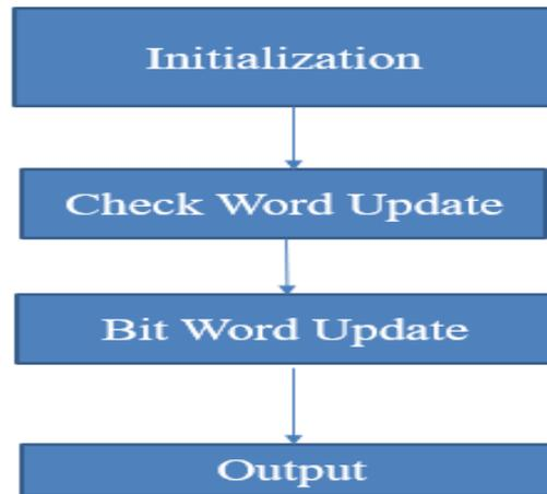
**Fig. 7: Process flow of LDPC Decoder.**
