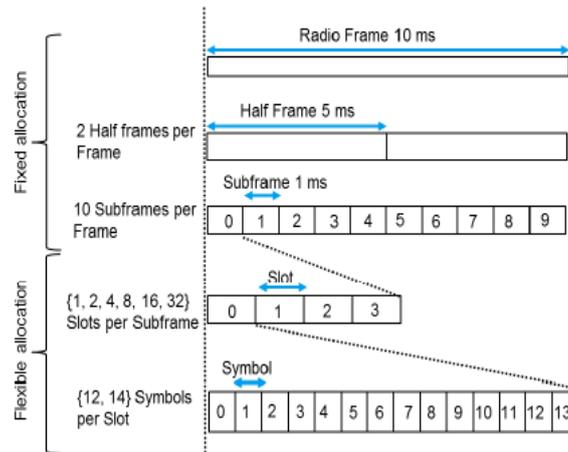
**Fig. 3: Frame Structure of 5G NR Technology.**
