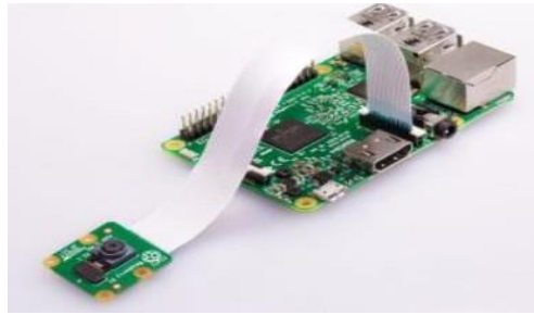
Figure 2: Raspberry Pi and Pi camera interfaced.
