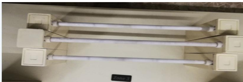
Figure 4: The three phases R, S, T and load.
