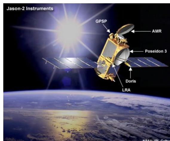
Fig. 3: Jason 2 Satellite, www.bing.com/images .
