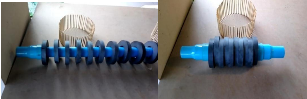
Figure 2.1: Magnets Before And Glue Is Applied.
