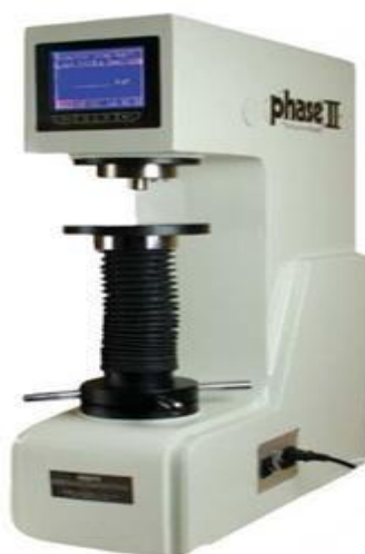
Fig. 3.4 Digital Motorised Rockwell Fig. 3.5 Vickers cum Brinell hardness hardness Testing Machines testers.
