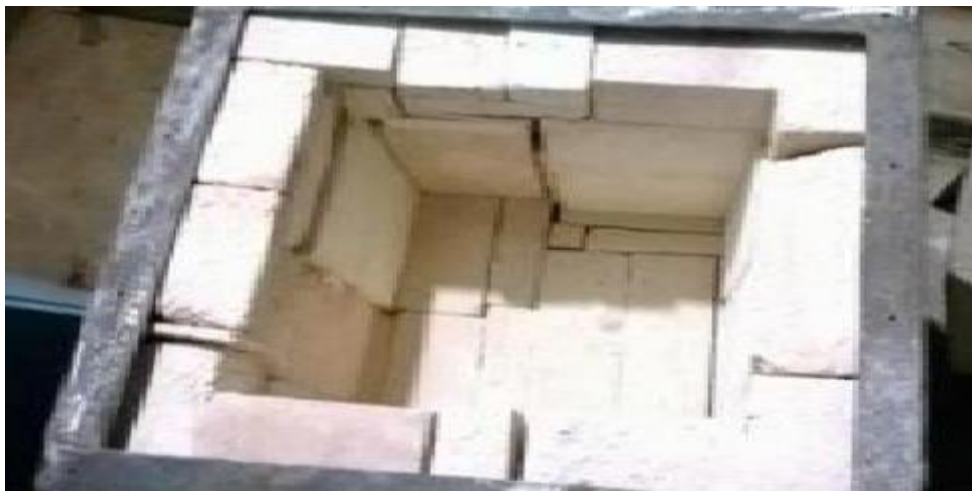
Fig. 4.5: Electric furnace frame with insulating materials.
