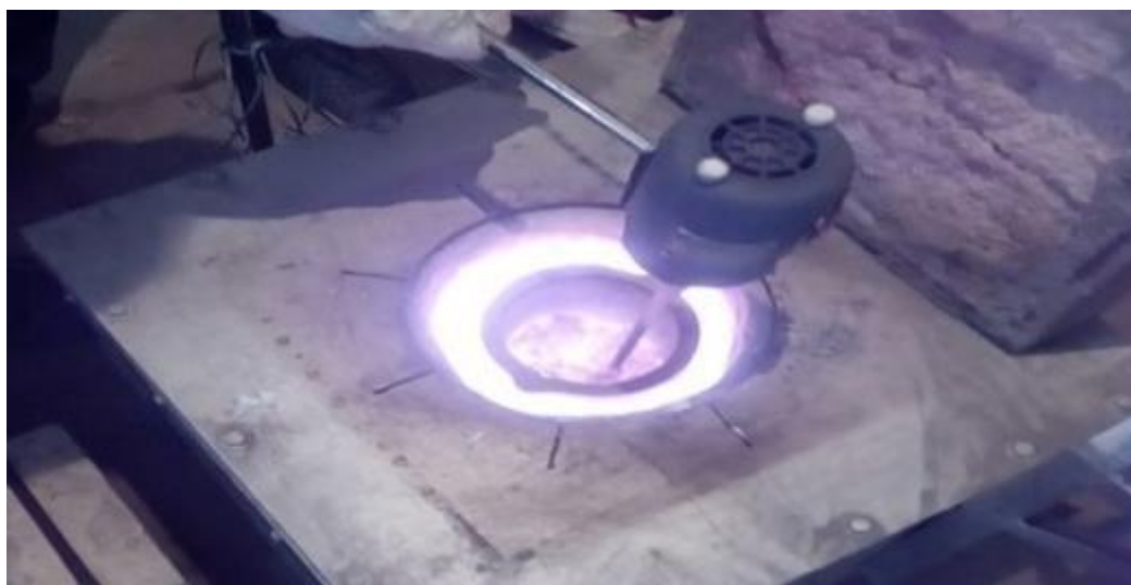
Fig. 4.12: Stirring of Reinforcements in molten composite.
