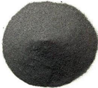
Fig 4.2 Iron powder 325 mesh
