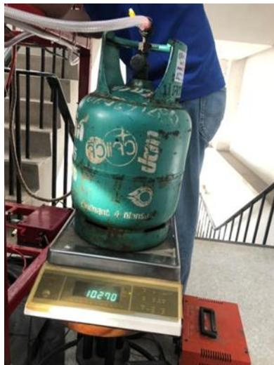
**Figure 4: LPG fuel consumption measurement.**
