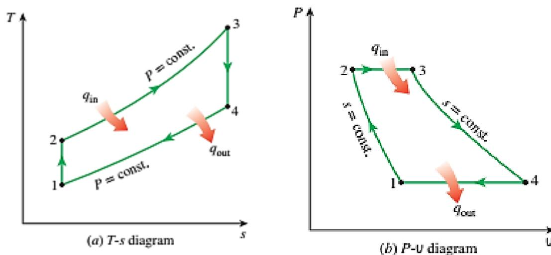
**Figure 2: T-s and P-v diagrams for the ideal Brayton cycle.**<sup>[2]</sup>
