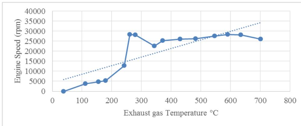
Figure 6: Motorspeed versus exhaust gas temperature data measurement.
