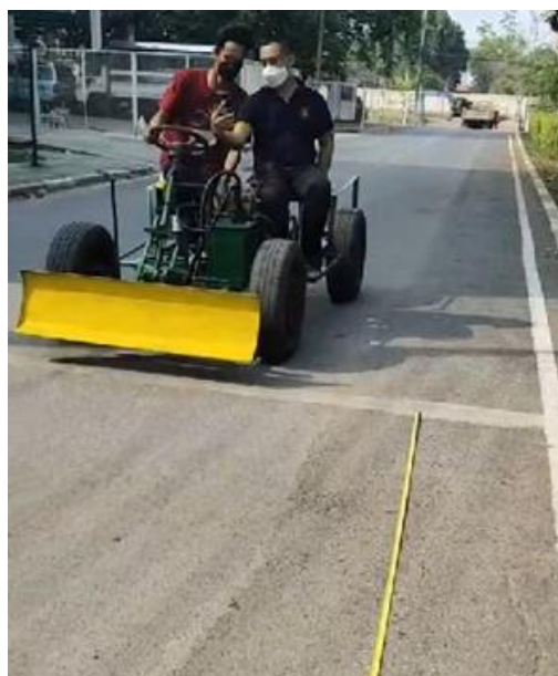
Figure 12: Testing to catch the braking distance.
