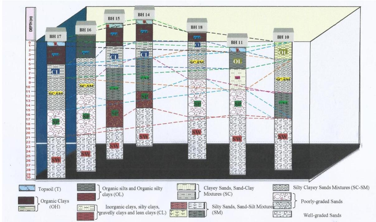
Figure 5c: Schematic Fence Diagram showing the Borings in Zone C.
