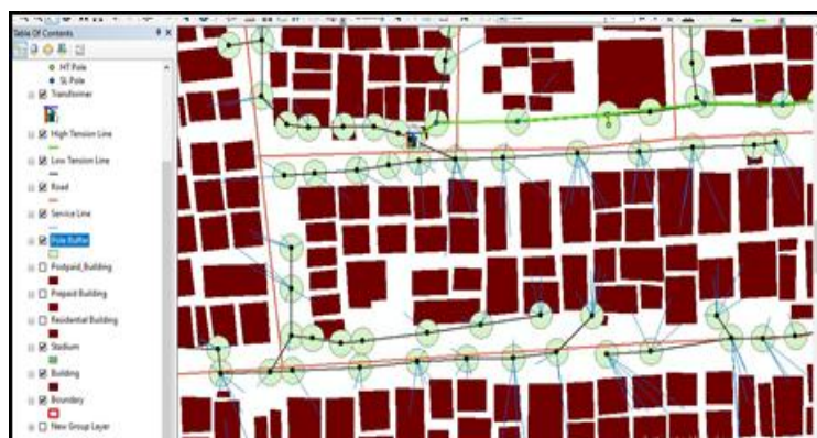
Figure 5: Diagram showing buffered electric poles by 6.0m.
