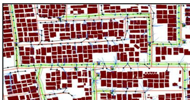
Figure 12: Diagram showing buffer of high tension lines by 9.0m.
