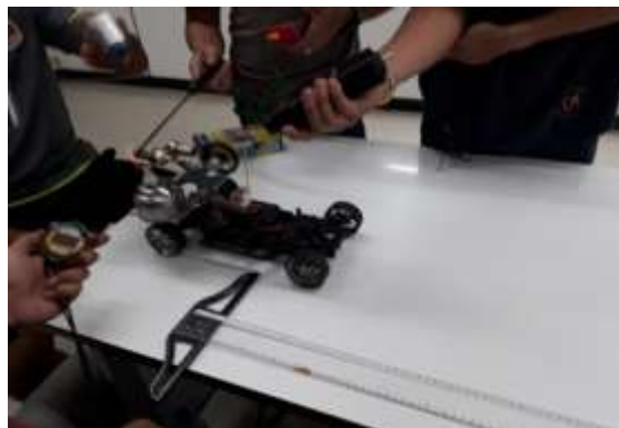
Figure 8: Testing the Stirling Engine-Powered Vehicle Using Alcohol as Fuel.
