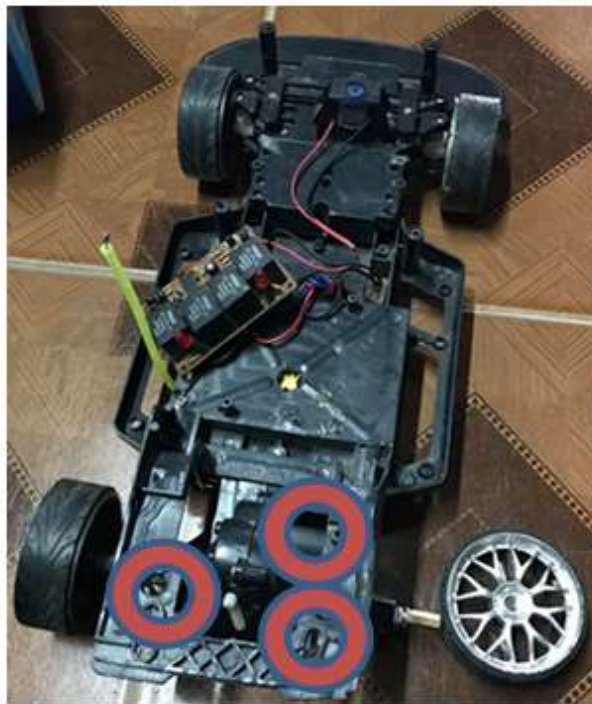
Figure 3: Installed drive belt and hole screw drilled.
