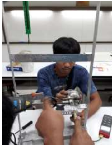
Figure 7: The Stirling engine is installed on the dynamometer testing stand, utilizing alcohol as fuel.
