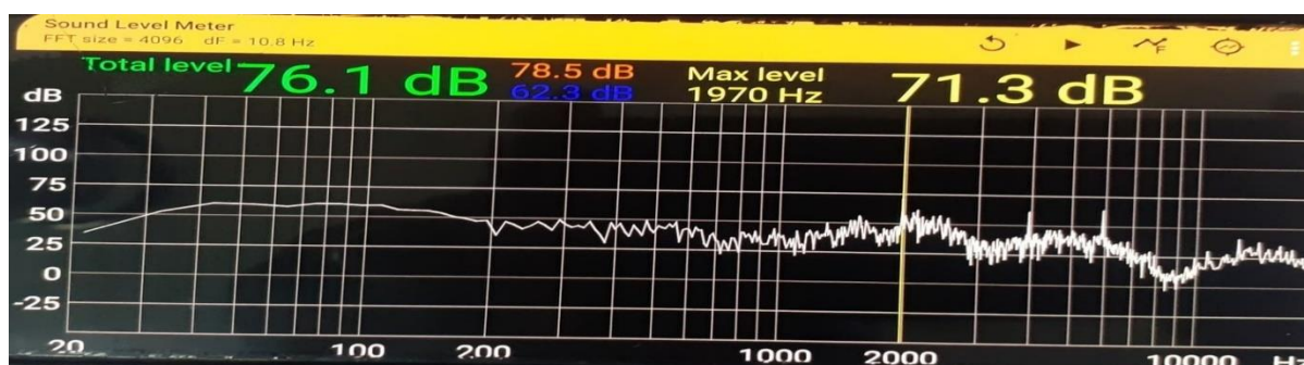
Figure 12: Sound Profile of Electric Motor using Direct Online Starter.
