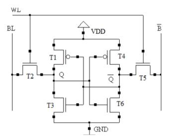
Fig. 1.1: Circuit diagram of SRAM.
