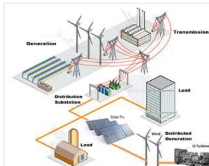
Figure 1: Distribution System with Distributed Generation. [7]
