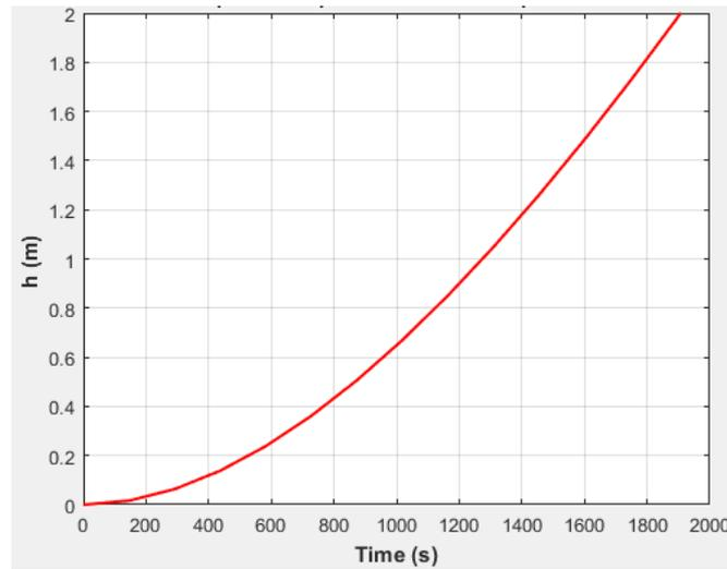
**Figure 2: Step response tracking of the LNG level.**
