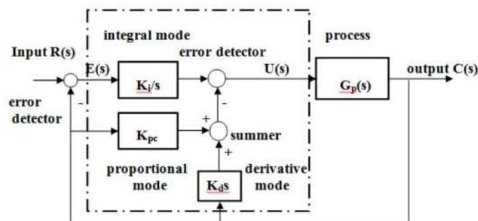
Figure 4: Control system using an I-PD controller.<sup>[23]</sup>
