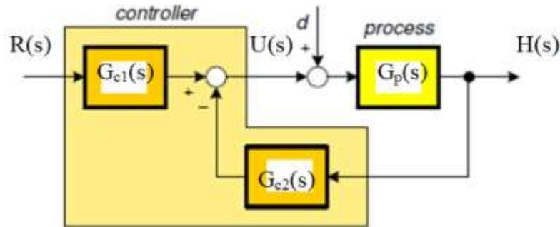
Figure 6: Structure of a 2DOF controller.<sup>[25,28]</sup>
