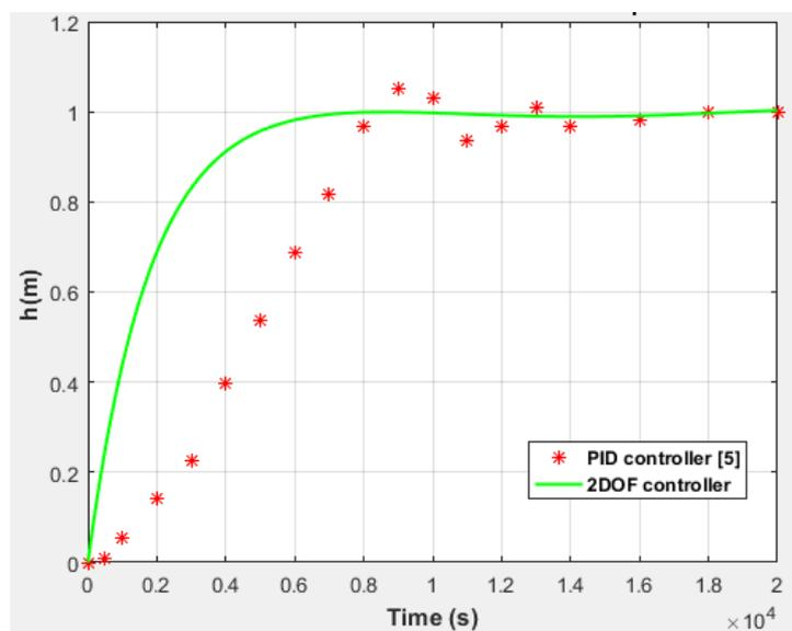
**Figure 9: Step response tracking with 2DOF and PID controllers.**
