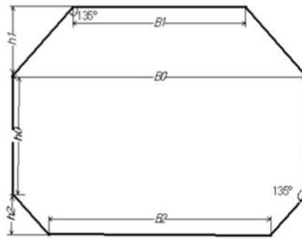
**Figure 1: Cross-section of LNG Dapeng Sun tank No.2.<sup>[9]</sup>**
