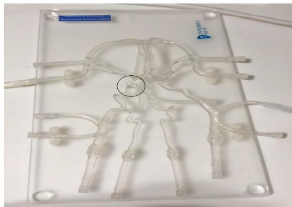
Figure 03: Overall Setup of In-Vitro Neurovascular Simulation Model with Aneurysm for Deployment of Nitinol Flow Diverter.
